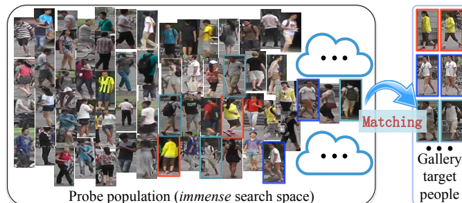
Fig. 1: Large scale open-world person re-identification aims to re-identify a gallery target person (right box) among an inherently immense probe search population (left box). This is due to no prior knowledge about the search space boundary and many non-target people are inevitable in deployments. Target identity is indicated with coloured bounding box.
