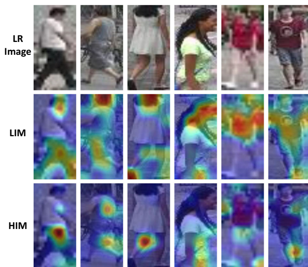
Fig. 5 A large difference in the class activation maps derived by low-resolution specific identity mapping (LIM, second row) and high-resolution specific identity mapping (HIM, third row) suggests that the learning module could extract different complementary appearance feature information from the LR and HR person images
